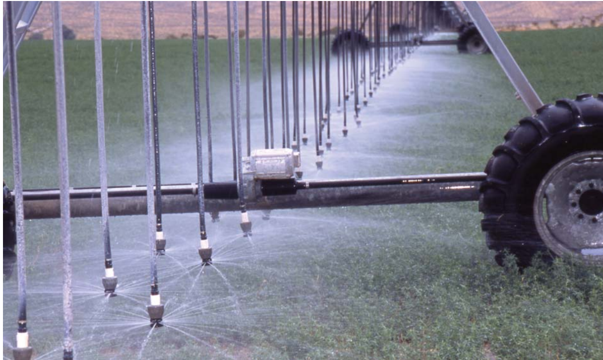
A low-energy, precision watering device irrigates an alfalfa field in Newberry Springs, Calif., part of a SARE grant project teaching farmers how to use soil moisture sensors to conserve water. – Photo by Ron Daines
